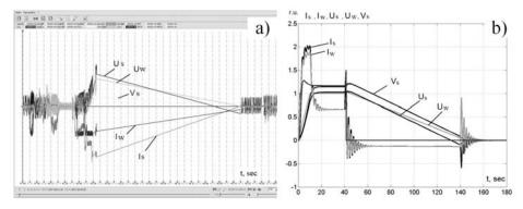
Fig. 9. Average CRM electromechanical processes (a), simulation results (b) in case of a strip break
