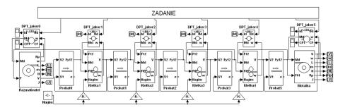
Fig. 10. Multi-mass electromechanical system of the four-stand cold rolling mill model
