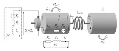
Fig. 2. Two-mass DC motor electric drive model with independent excitation
