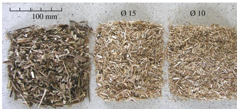
Fig. 2 Shredded Mushroom Shoots: from the right grinded on the ax cutter, then ground on a mill with Ø15 mm and Ø10 mm sieve Source Own elaboration
