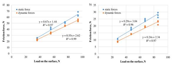
Fig. 2. Examples of friction force sample for alder wood chips,  $l_z = 15$ mm: a – humidity 52.9 %; b – humidity 13.1 %
