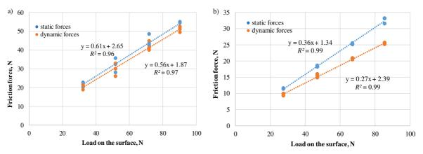
Fig. 3. Examples of friction force sample for robinia wood chips,  $l_z = 15$ mm: a - humidity34.4 %; b - humidity 11.5 %
