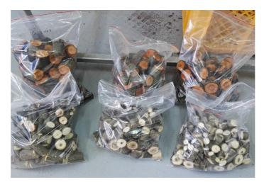
Fig. 1. Samples prepared for testing, in foreground black locust, on the second alder
